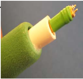
Fig 1) Use 50 ohm conversion kit to short one probe tip to Twin-Ax probe shield. Instructions: http://www.gigaprobes.com/usingaccessories/50ohmprobesetup.html
