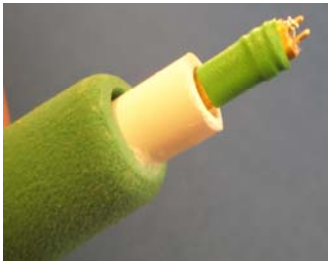
Fig 20) Use 50 ohm conversion kit to short one probe tip to Twin-Ax probe shield.
