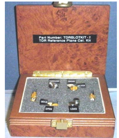
Fig 17) DVT Solutions, LLC TDRSLOTKIT – Qty two (2) each: Female SMA Short, Load, Open, Through). Contains optional Qty two (2) Male 50 ohm loads for TDR module calibration
