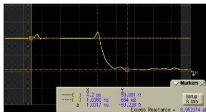
Fig 14) GigaProbes™ tip across SHORT pad.
