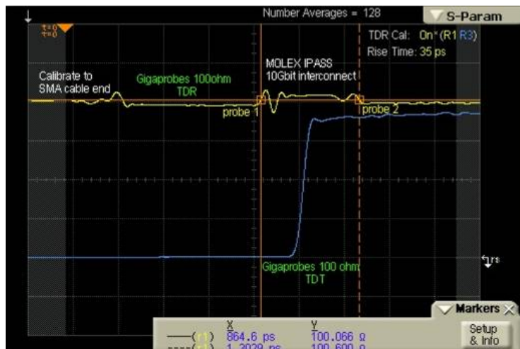
Fig.28) Plot taken from Agilent 86100C DCA-J mainframe shows the differential TDR impedance and TDT SAS/SATA connector measurements. Establish TDR reference plane at the SMA connector end. Establish measurement plan, place cursor #1(solid line) where the probe connects to the PCB and use cursor #2 (dotted line) to make Impedance measurements.
