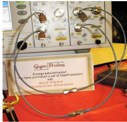
Fig 16) Connect Ch1 & Ch3 and Ch2 & Ch4 when required for the THROUGH calibration
