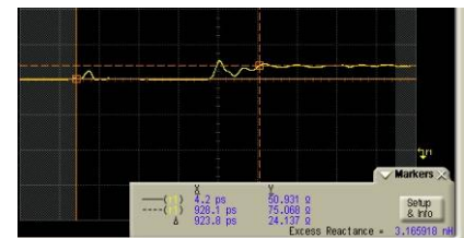
Fig 15) GigaProbes™ tip across 75 ohm pad.
