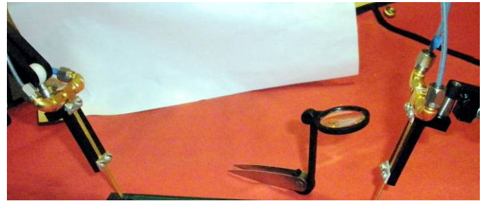
Fig. 35) Close up of the GigaProbes® connected to each end of the Test PCB coupon. Use the 5x micro lens to carefully place the probe on the test pads.
