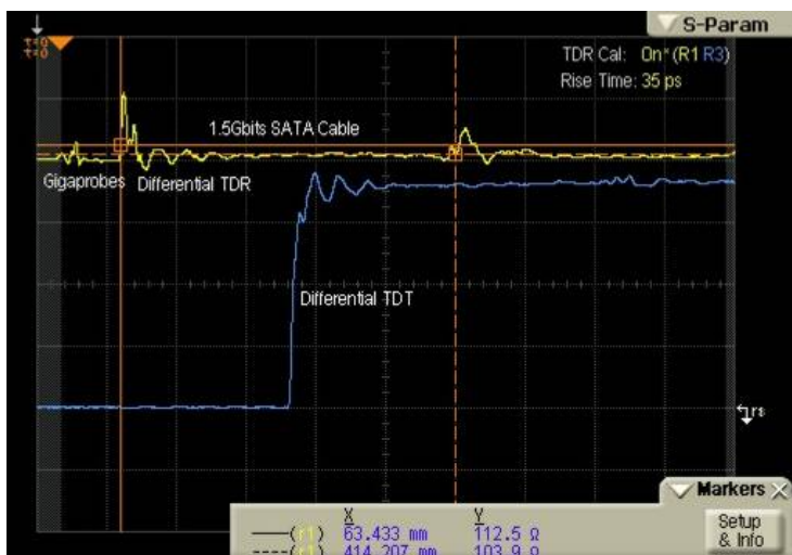
Fig. 32) Plot taken from the Agilent 86100C DCA-J mainframe shows differential TDR impedance and TDT SATA cable measurements. TDR reference plane established at the SMA connector end. To establish a reference plane, cursor #1 (solid line) is placed where the probe connects to the PCB and use cursor #2 (dotted line) to make impedance measurements.
