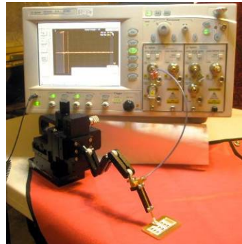
Fig 3) Use the Agilent Part# N1020A-K05 Calibration Substrate for the 50 ohm & Short measurement to establish TDR reference plane at probe tips
