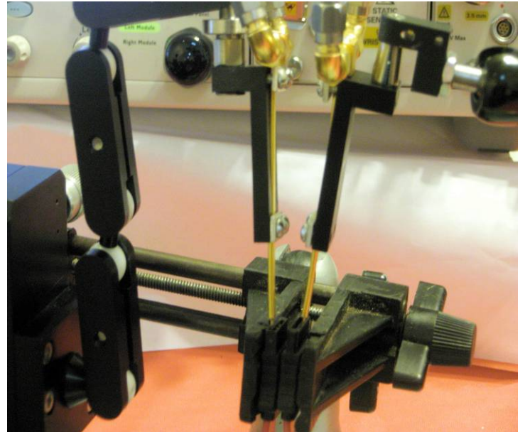
Fig. 31) SATA cables connectors being held in the vertical vice. Both GigaProbes™ are held in place using probe manipulators.
