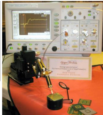
Fig21) GigaProbes® installed in a probe manipulator to probe a device package held by a vacuum chuck. Results display in Fig 24.
