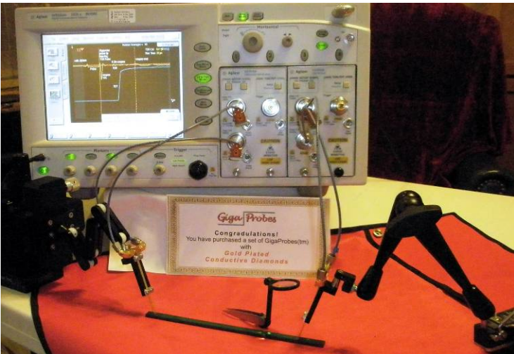
Fig. 34) Full setup for hooking up the GigaProbes® to make Differential Impedance and two port (SDD11/21) and return and insertion loss measurements on a test coupon. The display on the Agilent 86100C DCA-J mainframe shows the TDR/T plots.
