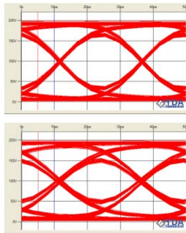
Figure 20. Modeled eye diagrams with and without connectors.
